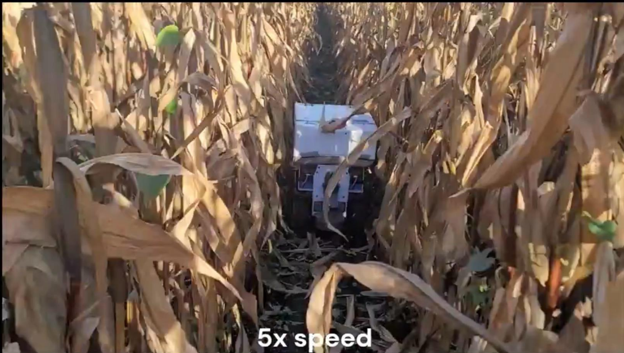
Under-canopy cover crop planting robot navigating with CropFollow++
